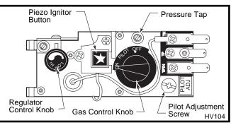
Fig. 47 RN & RP valve control.
